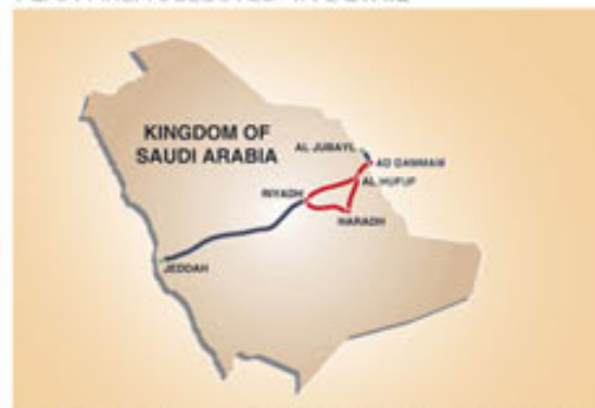
LANDBRIDGE PROJECT IS A MIXED TRAFFIC LINE WITH A PLANNED TOP SPEED OF 350 KM/H (WITH THE ELECTRIFIED LINE) FOR PASSENGER TRAINS AND 160 KM/H
